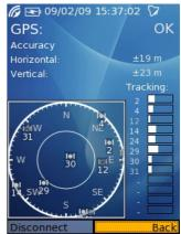
By pressing <code>Connect/Disconnect</code> you can create or interrupt the connection with GPS manually. By interrupting the connection temporarily, you can save the battery capacity significantly if you are in a location with poor signal for a longer period of time (status <code>no fix</code>), such as some buildings, the underground, etc. You can also disconnect from GPS directly by pressing <code>Stop/Start</code> in the menu (see Stop/Start).
